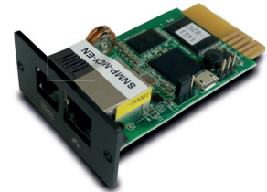
Option card: EMD (Environmental Monitoring Device)
